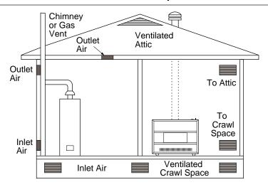
Figure 14 - Ventilation Air from Outdoors
